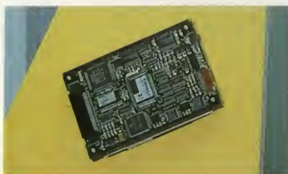
"GigaFix", a miniature internal 20 MB hard disk for the Amiga 500 manufactured by Gigatron, developers of a portable Amiga.
